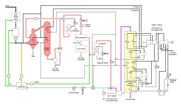
Fig. 1: IGCC Plant schematic layout
