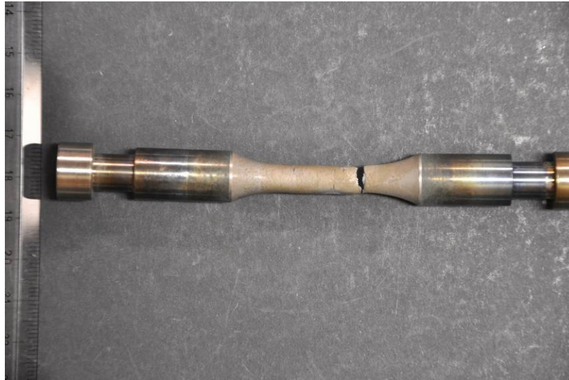
Figure 51 – R262-6 broken specimen after 665 cycles in TMF test
