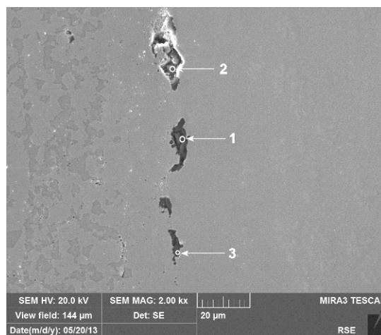
Figure 83 – Precipitates and defect at the interface between bond coat and base metal of specimen R262-3
