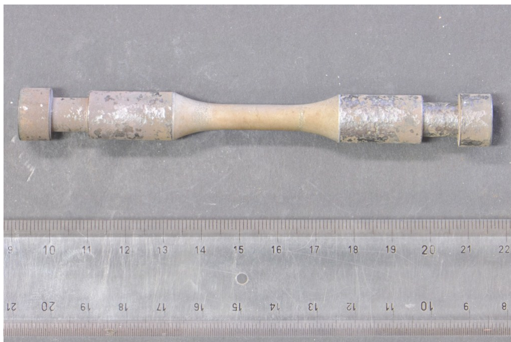
Figure 79 – Aspect of specimen R262-3 after ageing in air with 20% steam
