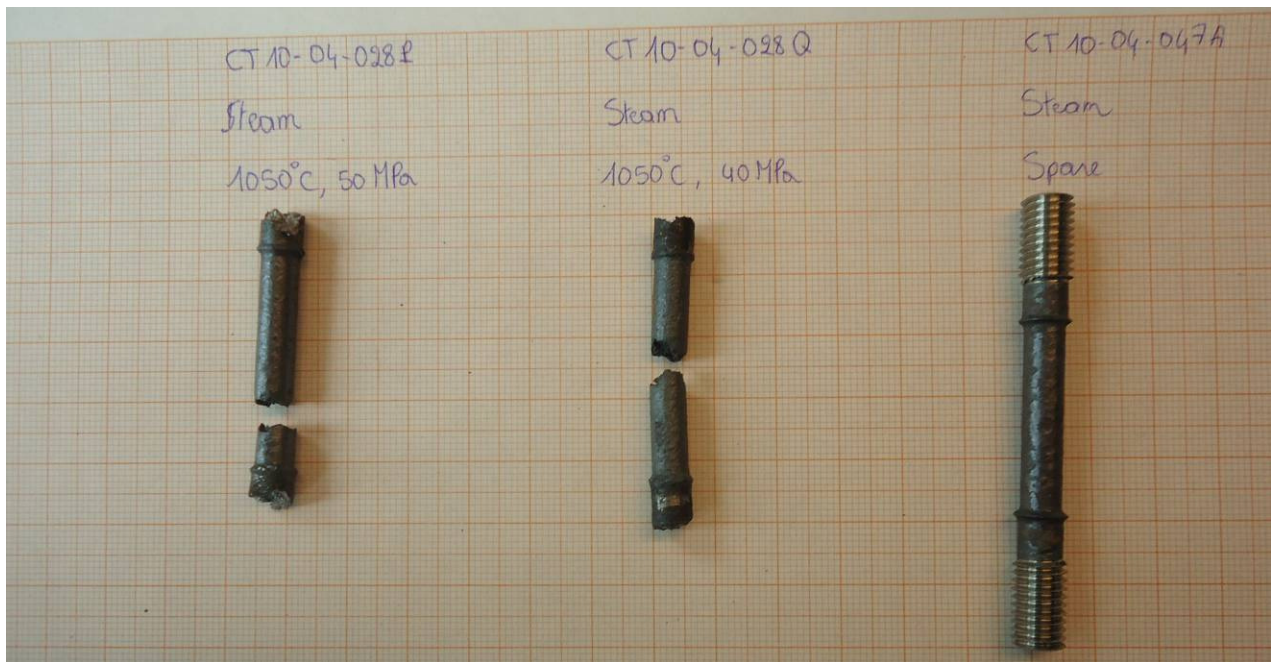
Figure 124: Creep samples of “Uncoated as received René 80 pre-aged in air+20% steam (1000hrs at 1000°C) after creep test till rupture at different test parameters. Sample on the right is not tested.
