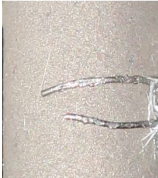
Figure 2 –TMF specimen surface with \varnothing 0.6 mm thermocouple wires
