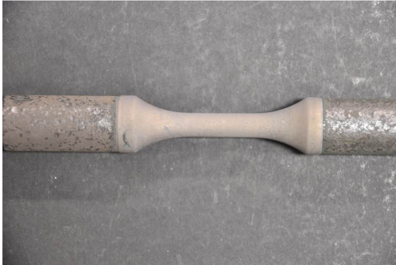
Figure 11 - TMF specimen after ageing in air
