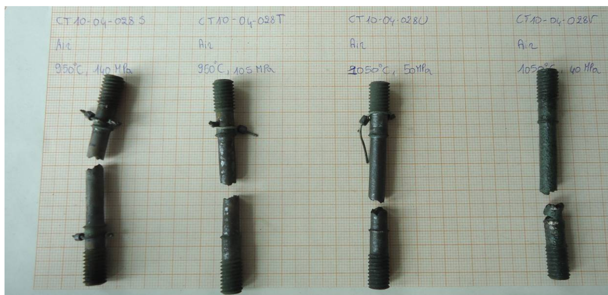
Figure 123: Creep samples of "Uncoated as received René 80 pre-aged in air (1000hr, 1000°C) after creep test till rupture at different test parameters.
