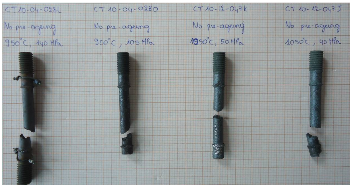
Figure 122: Creep samples of Uncoated as received René 80 after creep test till rupture at different test parameters.
