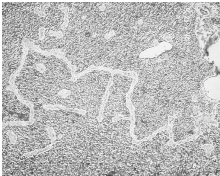
Figure 169 – Grain boundaries precipitates of a disc aged in air
