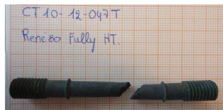
Figure 119: Creep SAMPLE CT10-12-047T René 80 fully heat treated by Laborelec, tested at 950°C and 140MPa
