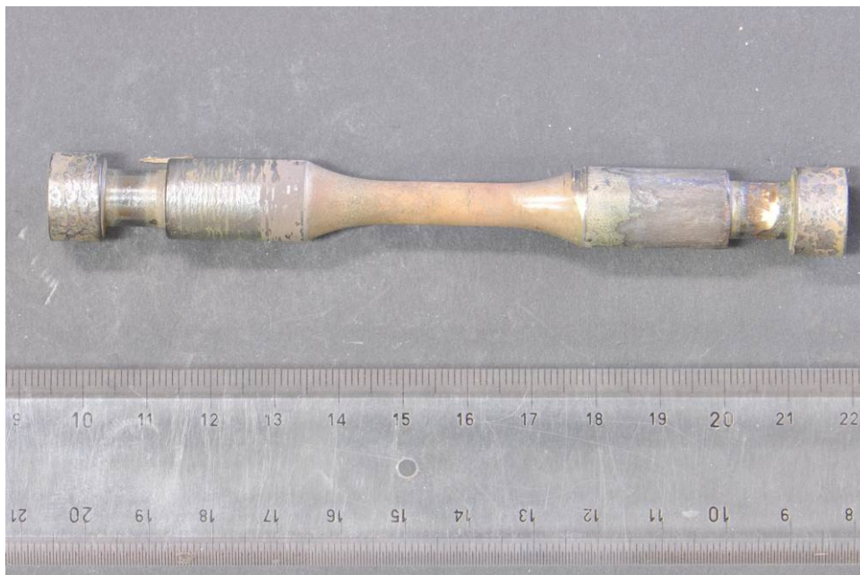
Figure 67 – Aspect of specimen R262-2 at the end of TMF test
