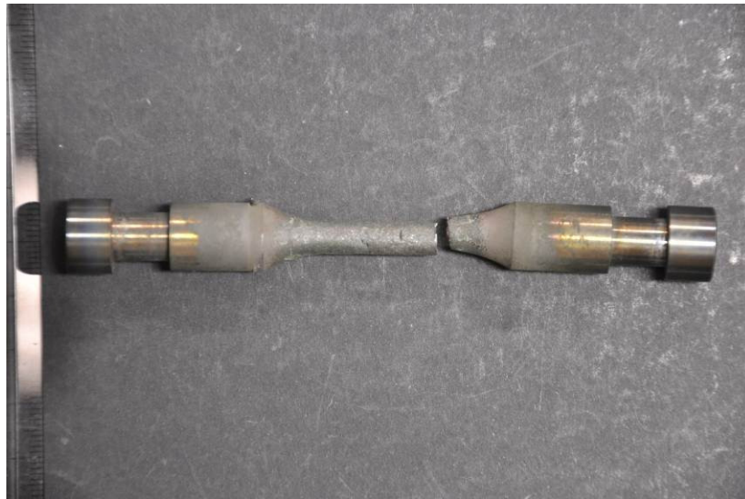
Figure 43 – R263-6 broken specimen after 1284 cycles in TMF test
