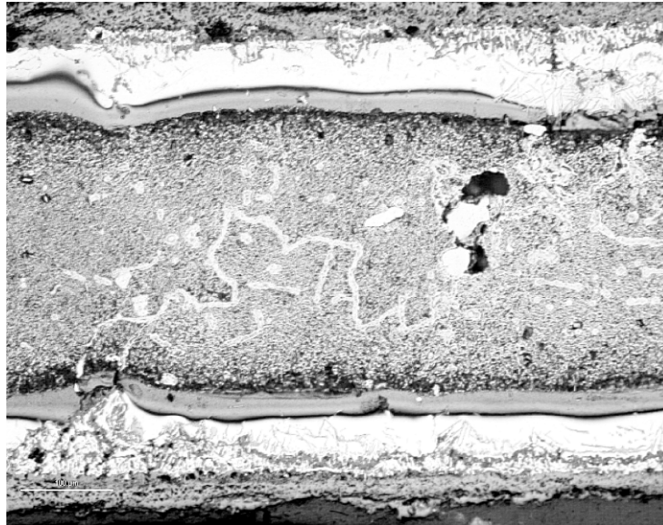
Figure 168 – Metallographic specimen of a disc aged in air
