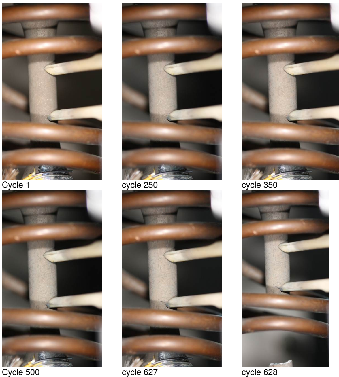
Figure 31 - Pictures taken at different cycles showing the growth of surface crack in gauge length for specimen R262-1 (coated Rene 80)
