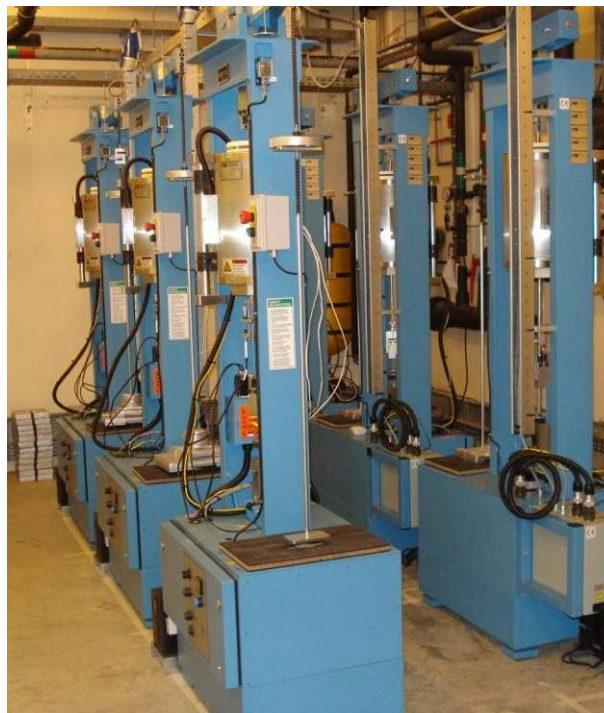
Figure 99 - ATS series 2320-MM dead weight single specimen lever arm creep testers with continuous strain monitoring.
