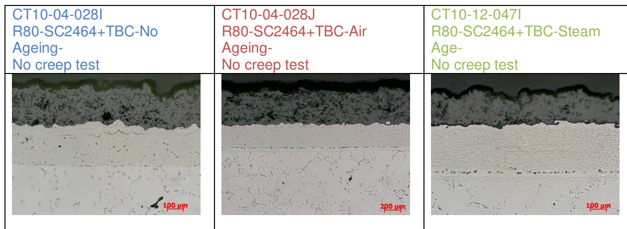
Figure 127: Microstructural features of “René 80 + SC2464 + TBC” without pre-ageing, with pre-ageing in air for 1000hrs at 1000°C and with pre-ageing in air + 20% steam for 1000hrs at 1000°C before creep test.
