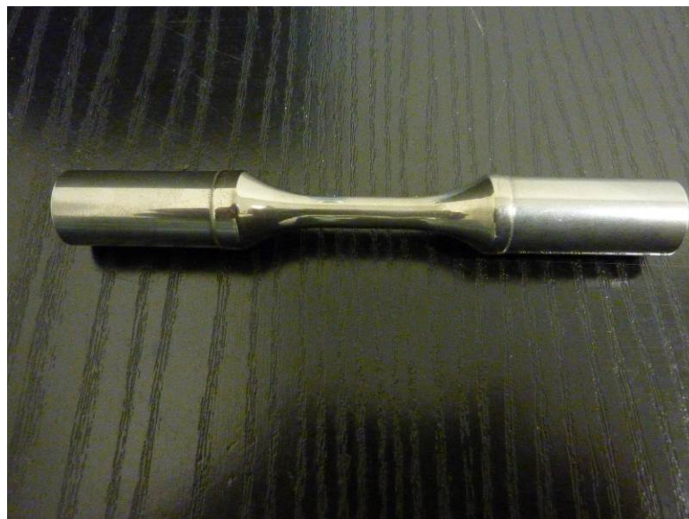
Figure 10 - TMF specimen after polishing up to 0.2 Ra in gauge length
