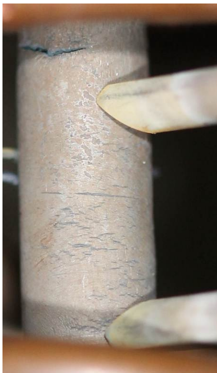
Figure 5 – Example of cracks in detail shown by front camera
