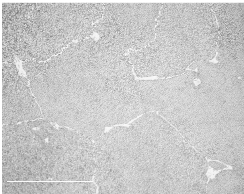
Figure 149 – LO micrographs of as received Rene 80
