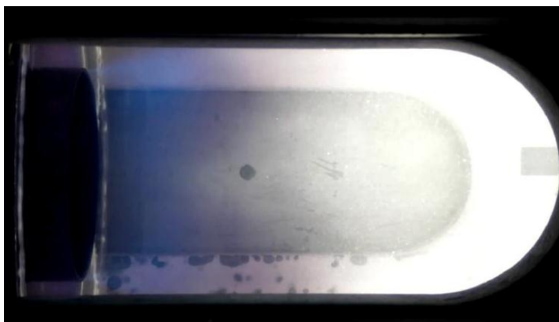
Figure 4: 19 th April. Configuration 3.2. 500 kWth axial syngas flame
