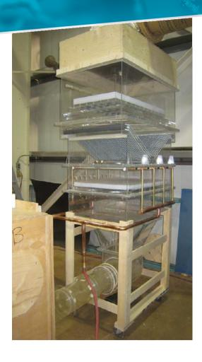
INNOVA Global was selected by LA Country to retrofit a CO \ NOx reduction system into an existing vertical flow HRSG system. The project required that Innova model the existing gas turbine & HRSG system to determine the optimal location to locate the new distribution grids, CO catalyst, ammonia injection and NOx catalyst components.
