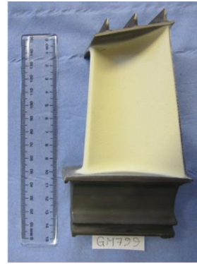
HVOF 2464 bond coating / standard TBC (reference)
