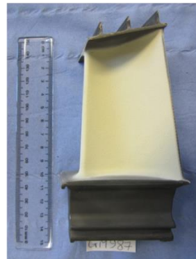
Figure 15 - Examples of coated blades prepared for exposure in the burner rig cascade
