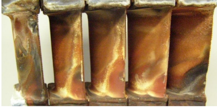
Figure 16 - First cascade blade cluster after 1000 hours operation: (a) upstream view and (b) downstream view
