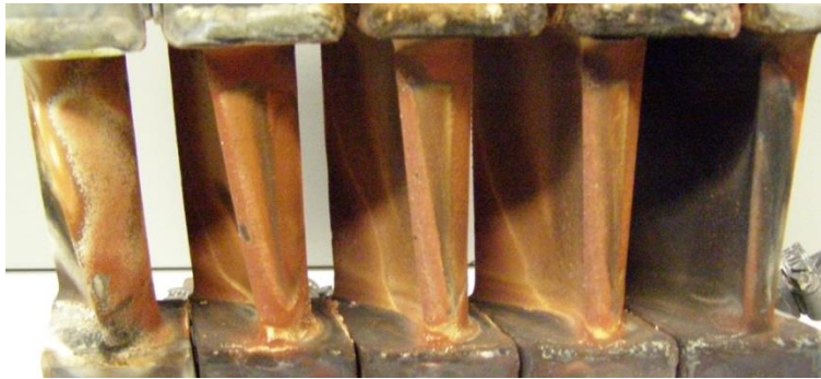
Figure 15 - Examples of coated blades prepared for exposure in the burner rig cascade
