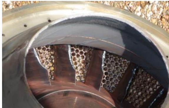
Fig.6 - Diagonal swirler blades after tests
