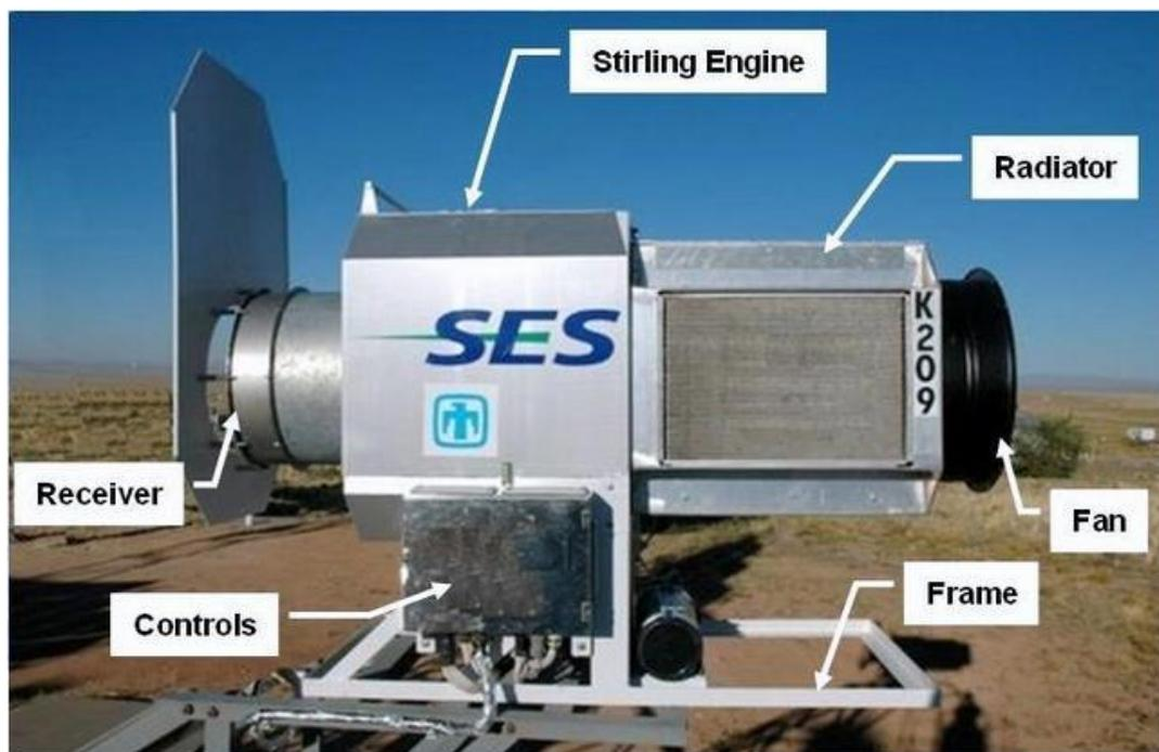
*Figure 17- SES kinematic Solar Stirling engine. It is a 4 cylinder, each with a 95cc displacement engine (4-95 engine) that evolved from the Philips engines of the 1960's*
