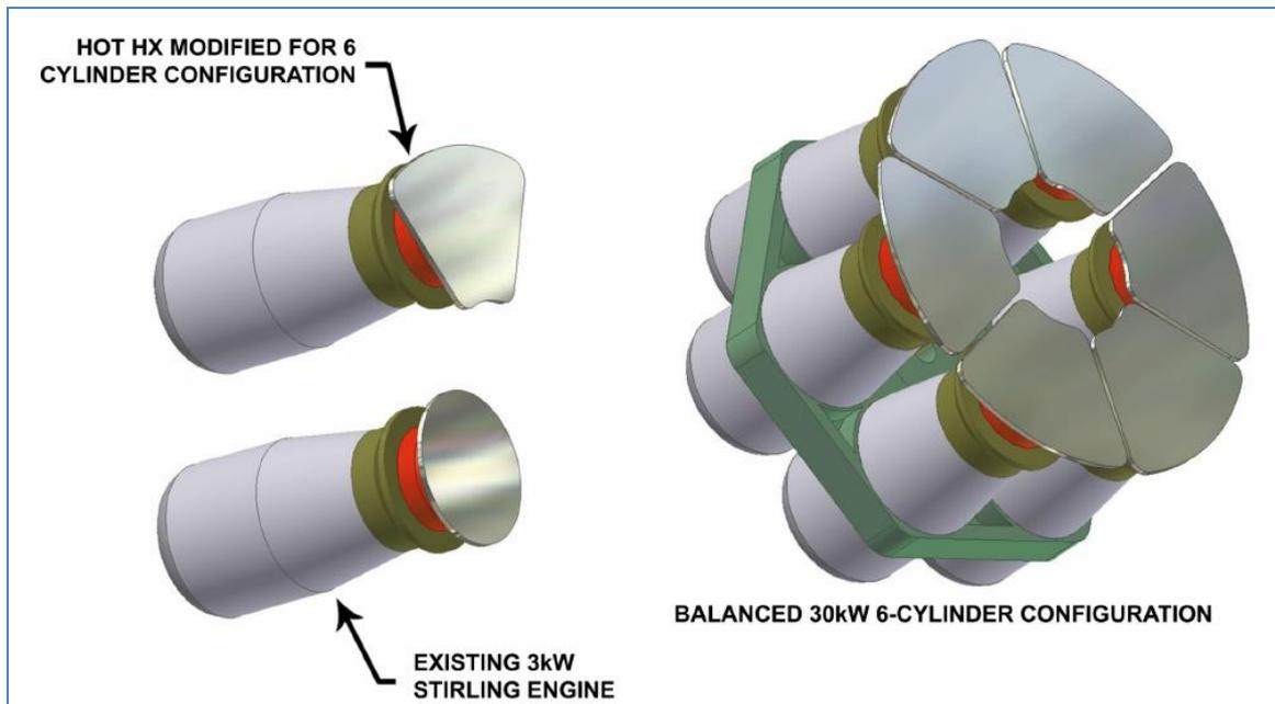
Figure 24 – Infinia 30 kWe 6-cilinder project
