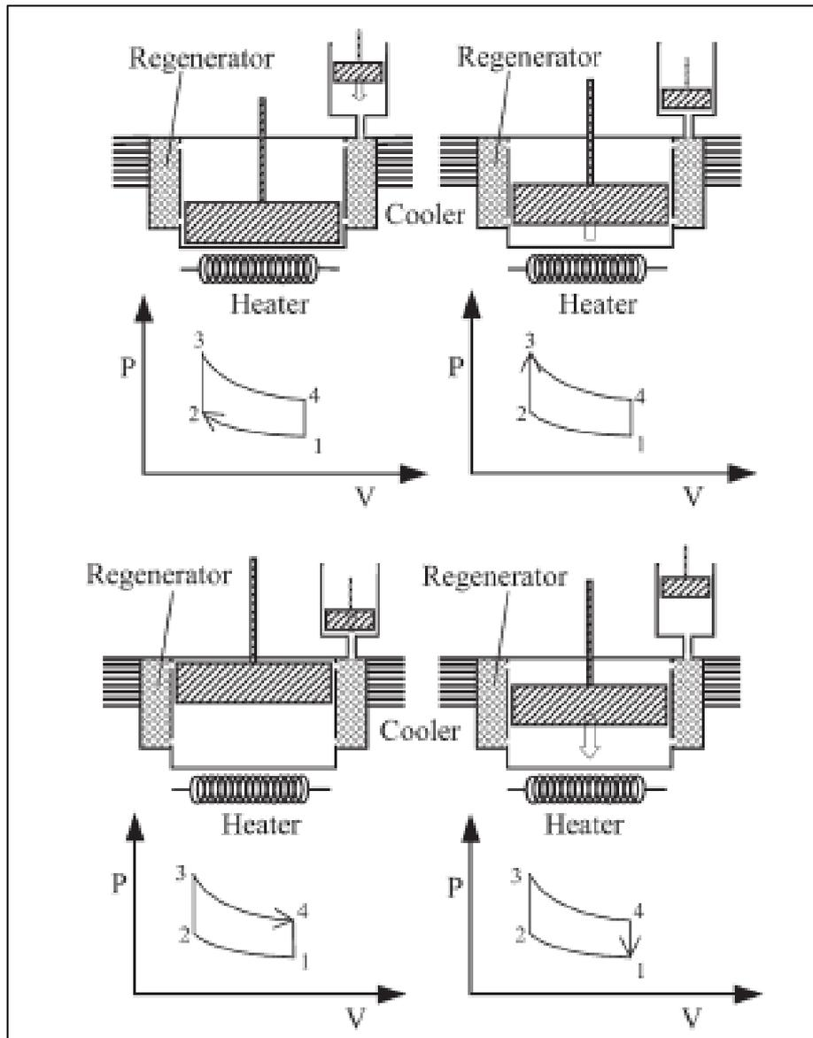
Figure 5 – Stirling engine operation [4]
