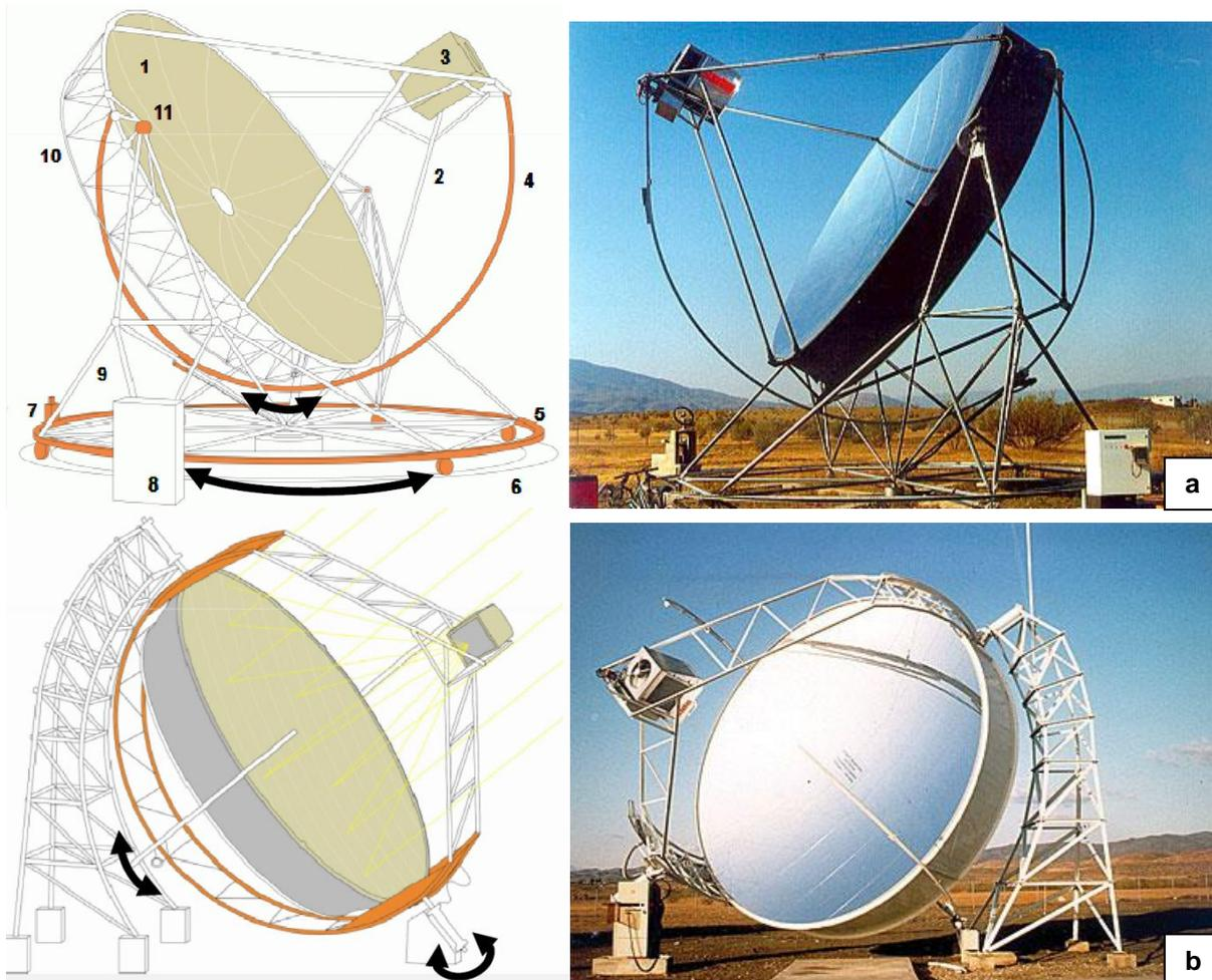
Figure 9 - a) Azimuth elevation Tracking System- Distal II Almeria 1996 b) Polar Tracking System- Distal I Almeria 1992
