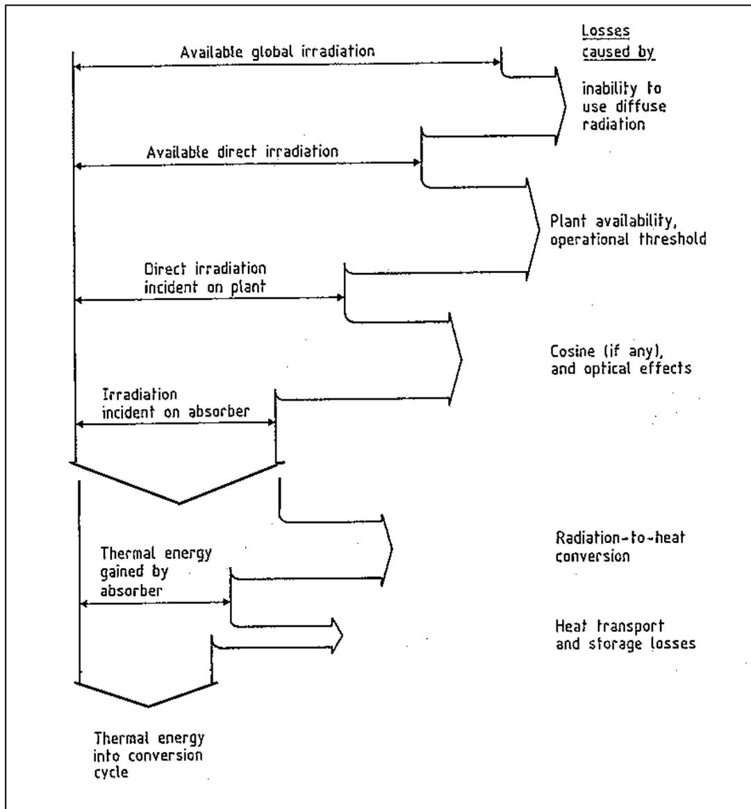
Figure 3 – Simplified Sankey Diagram for the Dish/Receiver System
