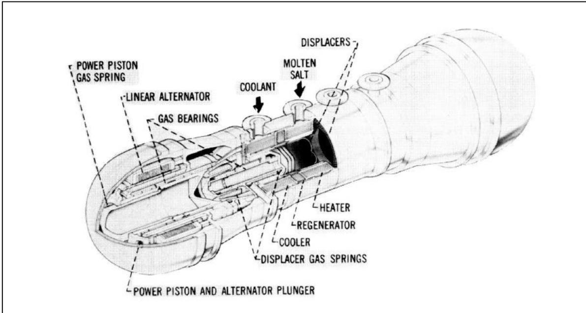
Figure 12 - 25 kWe Space Power Demonstrator Engine
