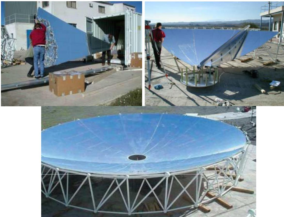
*Figure 8 - Segmented Dishes (Curved Glasses)[27]*
