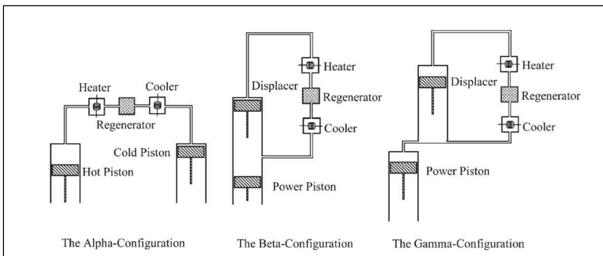
Figure 6 – Mechanical configurations for Stirling engines [4]
