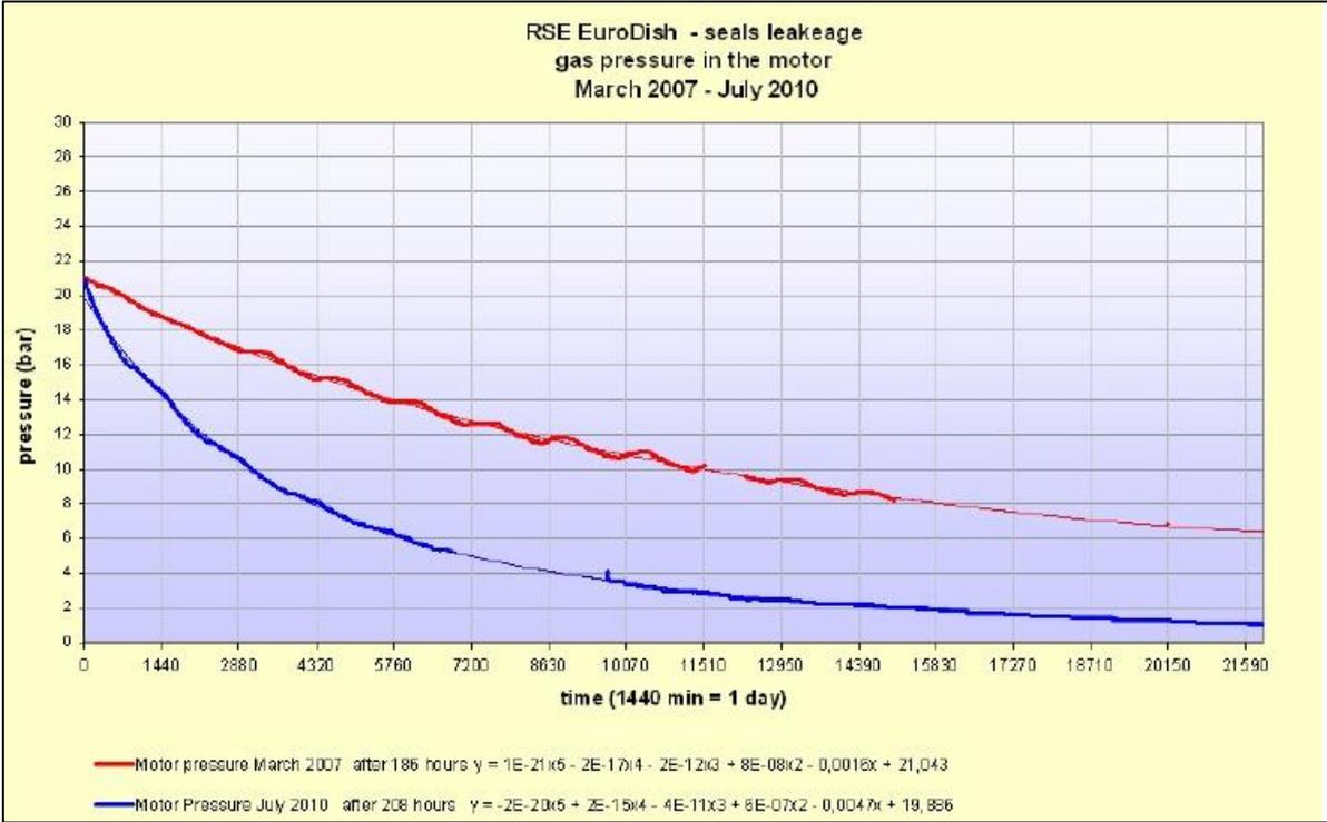
*Figure 31 – Eurodish – WF pressure in the engine [20]*
