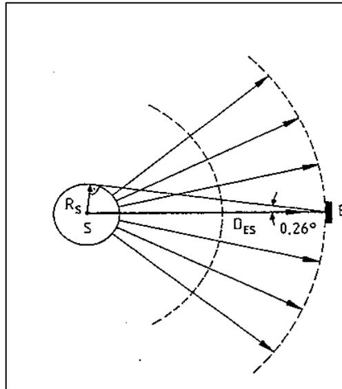
Figure 2 – Sun-Earth geometry. Assuming a Sun spherical surface of radius  $R_s$ ,  $E_{sc}$  is the Solar Constant observed at distance  $D_{ES}$  between Earth and Sun [1].
