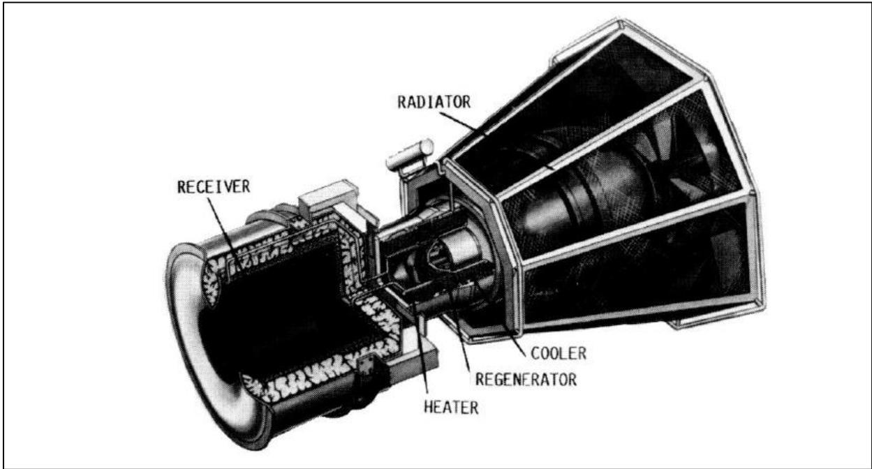
Figure 14 – Conceptualized Free-Piston Stirling engine conversion system
