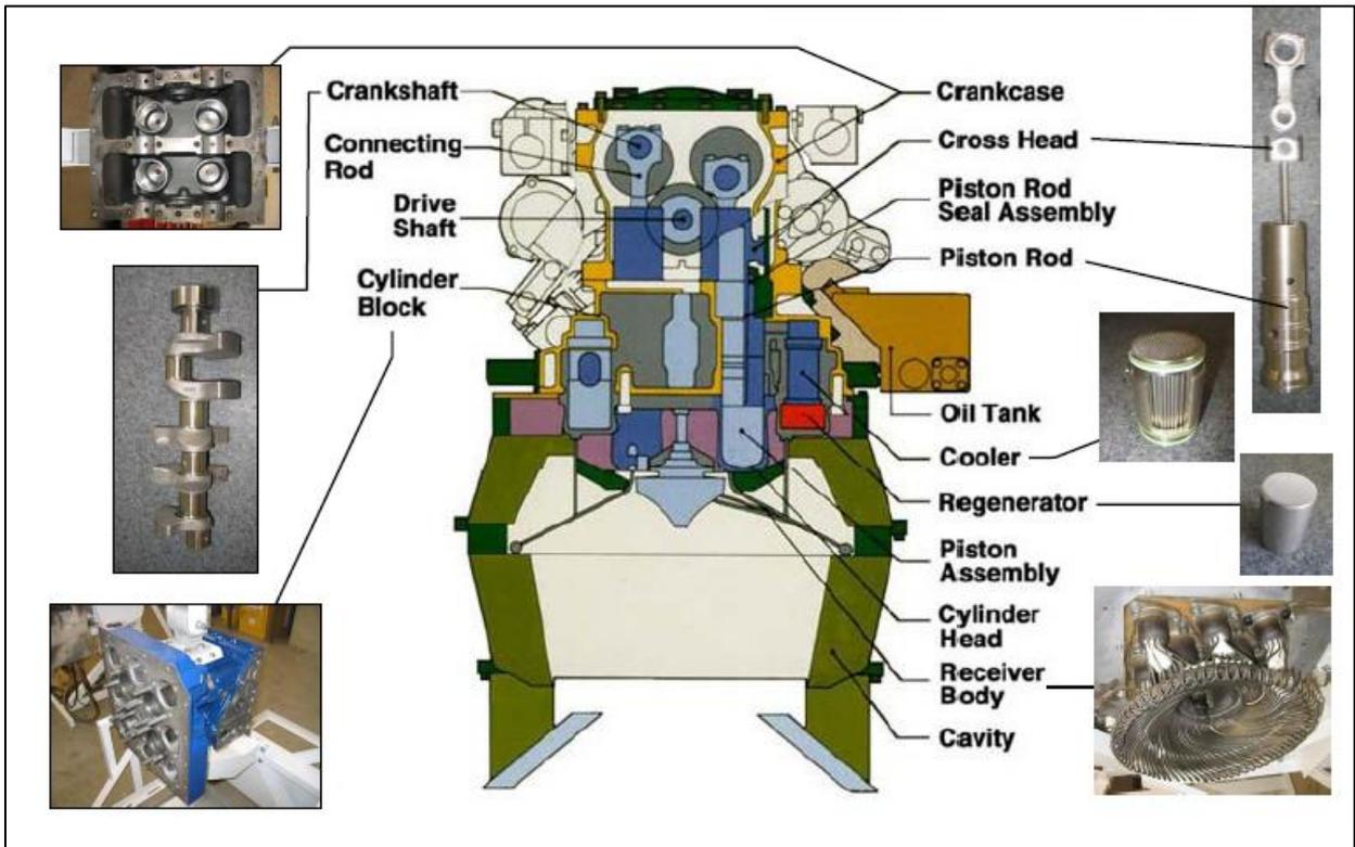
Figure 15 – Scheme of a kinematic engine and its main components
