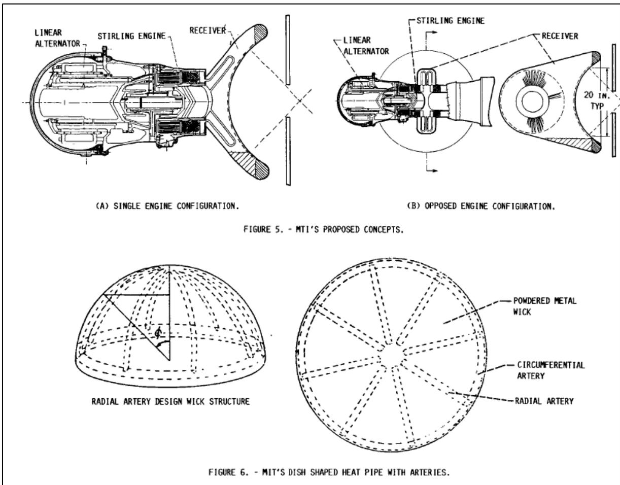
Figure 13- MIT's preliminary Dish-Stirling engine
