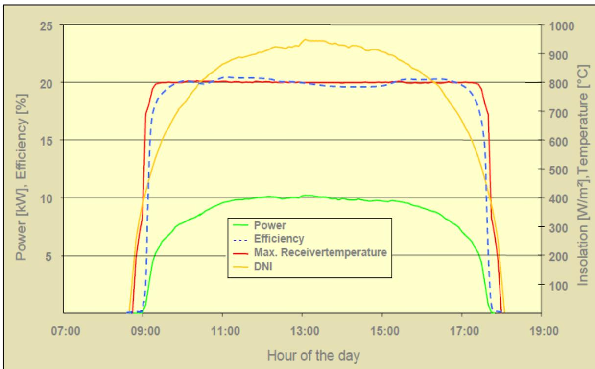
Figure 30 - Typical operation day in Spring (Measured on Feb. 2005 in Seville) [18]
