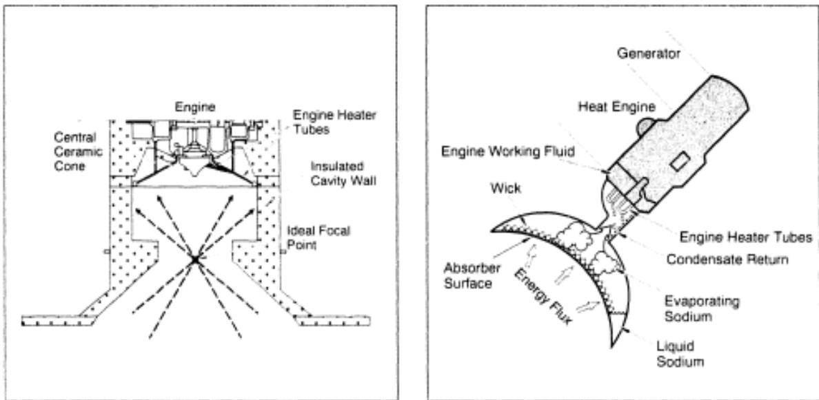
Figure 10 – a) Directly illuminated Tube Receiver b) Reflux heat-pipe Receiver
