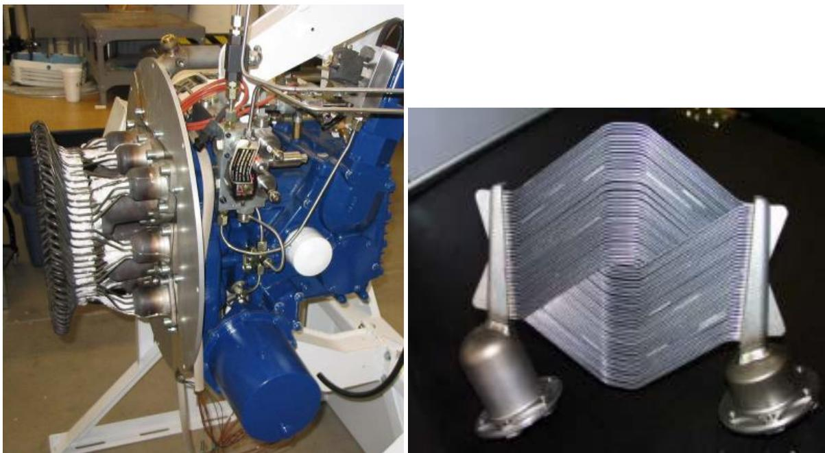
Figure 11 - Details of modern solar receivers for Solar Stirling engines
