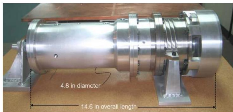
Figure 6: Brayton energy air bearing test configuration.
