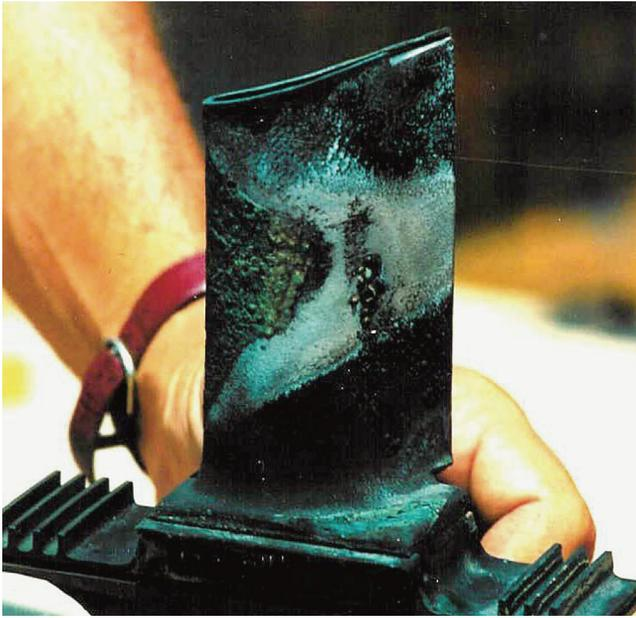
Figure 43. Hot Corrosion Blade Distress.
