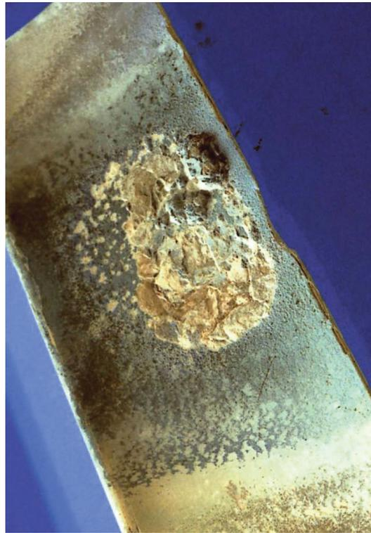
Figure 35. Example of Accelerated Surface Oxidation Caused by Vanadium in Heavy Fuel Oil.
