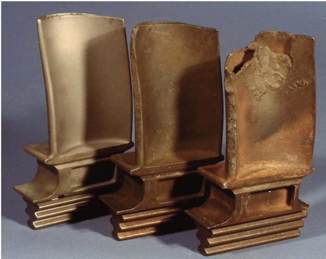
Figure 34. Sulfidation Corrosion on a 1970s Vintage Low-Firing Temperature Gas Turbine. Failure (Shown at Right) Occurred after about 1000 Hours Operation on Distillate Fuel Containing 2 ppm Sodium from Seawater Contamination.
