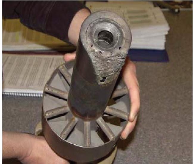
Figure 14 Flashback Damage. (Angello and Castaldini, 2004)
