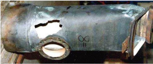
Figure 20. Transition Piece Damage Due to Dynamics.
