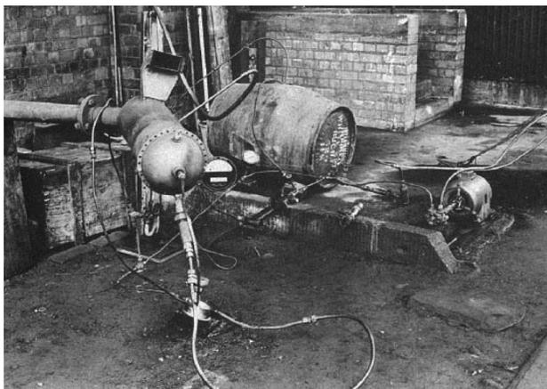
Figure 1. Whittle's Rudimentary Gas Turbine Combustor Test Rig, BTH Factory, Rugby, Circa 1936. (Meher-Homji, 1998).
