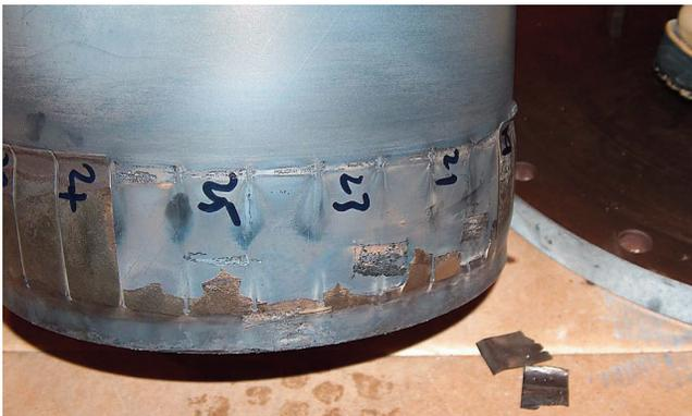
Figure 49. Damage on Liner Seals.
