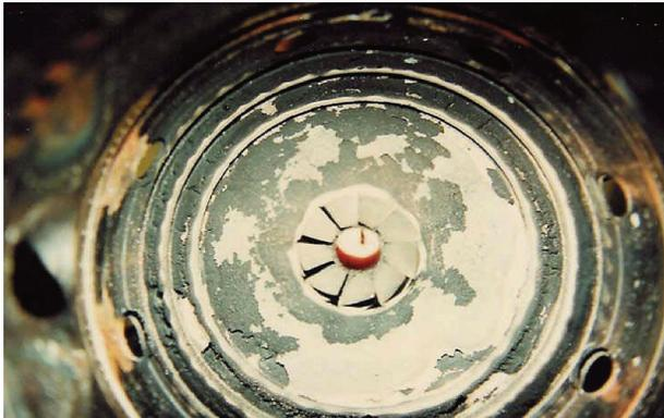
Figure 40. Coked Combustor Nozzle.
