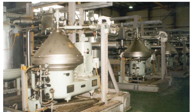
Figure 37. Two-Stage Centrifugal Fuel Treatment Plant for Heavy Fuel Oil. (Courtesy Westfalia Separator)
