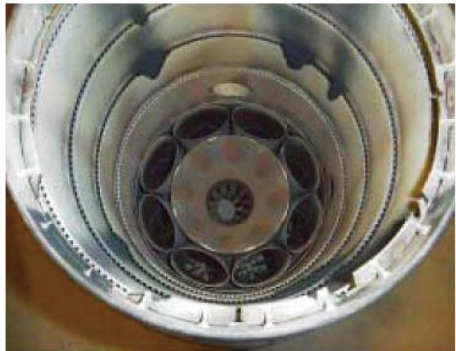
Figure 15 Flashback Damage. (Latcovich, 2002)
