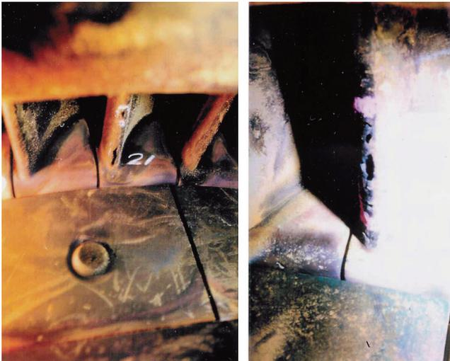
Figure 44. Nozzle Distress Due to Hot Corrosion.
