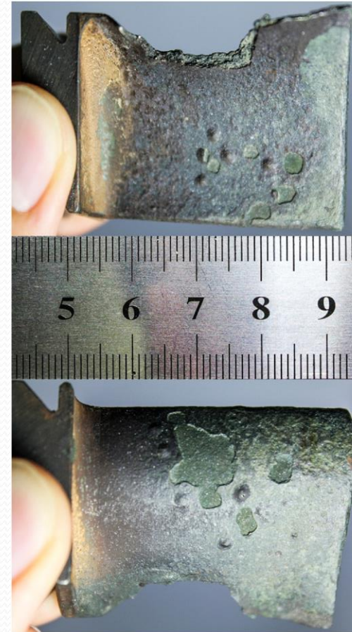
From: Salehnasab B, et al, Hot corrosion failure in the first stage nozzle of a gas turbine engine, Engineering Failure Analysis 60, pp 316–325, 2016 Slide: 17
