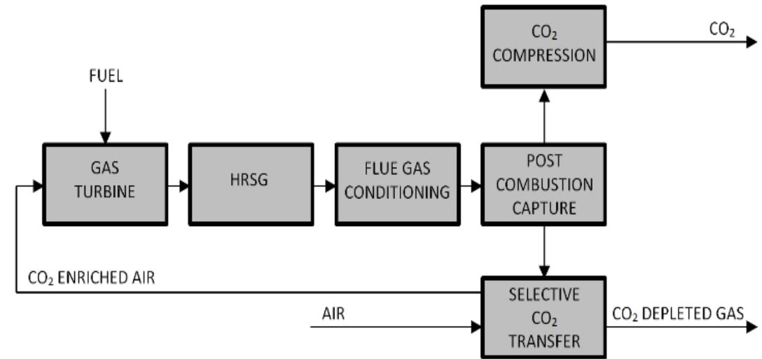
Process schematic of a series configuration S-EGR system, including extraction points and recycling loops of pure CO<sub>2</sub> and depleted exhaust gas (Merkel et al, 2013).
