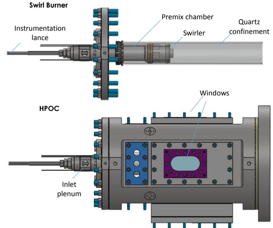
Schematic view of the swirl burner employed with the High Pressure Optical Chamber (HPOC)
