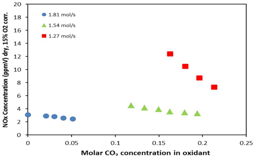
Normalised (dry 15%O<sub>2</sub>) NO<sub>x</sub> concentrations for each flow and CO<sub>2</sub> condition at 84 kW, 2.2 bar<sub>a</sub>.
