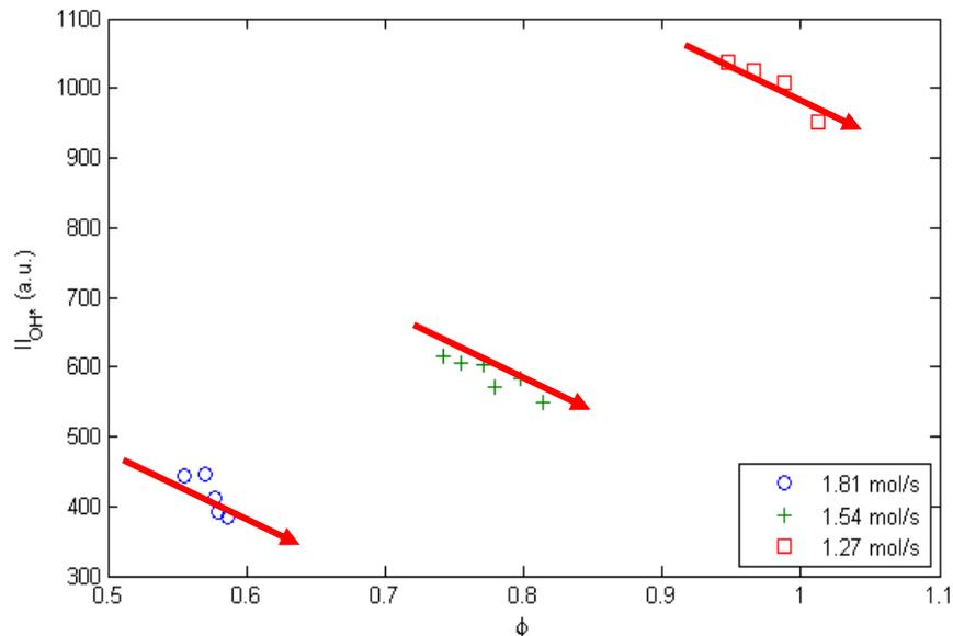
Average image chemiluminescence intensities for each flow and CO<sub>2</sub> condition at 84 kW, 2.2 bar<sub>a</sub>.
