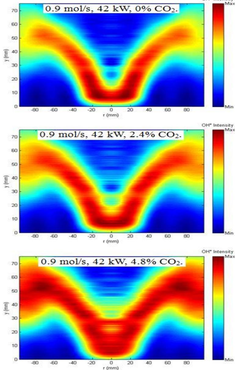
*Abel inverted chemiluminescence images at 42 kW, 1.1 bar<sub>o</sub> and 0.9 mol/s total flow for three  $\text{CO}_2$  concentrations in the inlet premix.*
