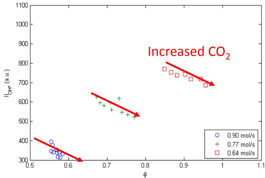
Average image chemiluminescence intensities for each flow and CO<sub>2</sub> condition at 42 kW, 1.1 bar<sub>a</sub>.
