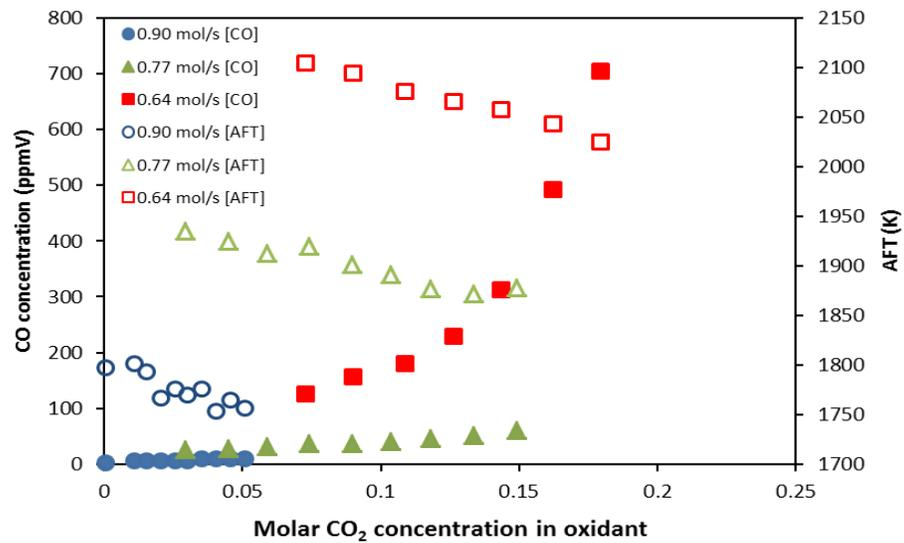
Measured CO concentrations and modelled AFT for each flow and CO<sub>2</sub> condition at 42 kW, 1.1 bar<sub>a</sub>.
