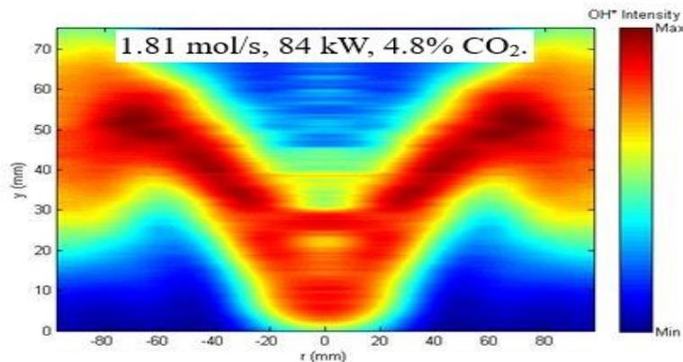
*Abel inverted chemiluminescence images at 84 kW, 2.2 bar<sub>0</sub> and 1.81 mol/s total flow for three CO<sub>2</sub> concentrations in the inlet premix.*
