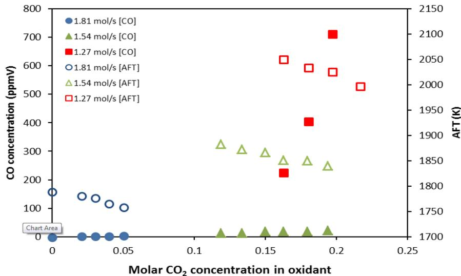
Measured CO concentrations and modelled AFT for each flow and CO<sub>2</sub> condition at 84 kW, 2.2 bar<sub>a</sub>.
