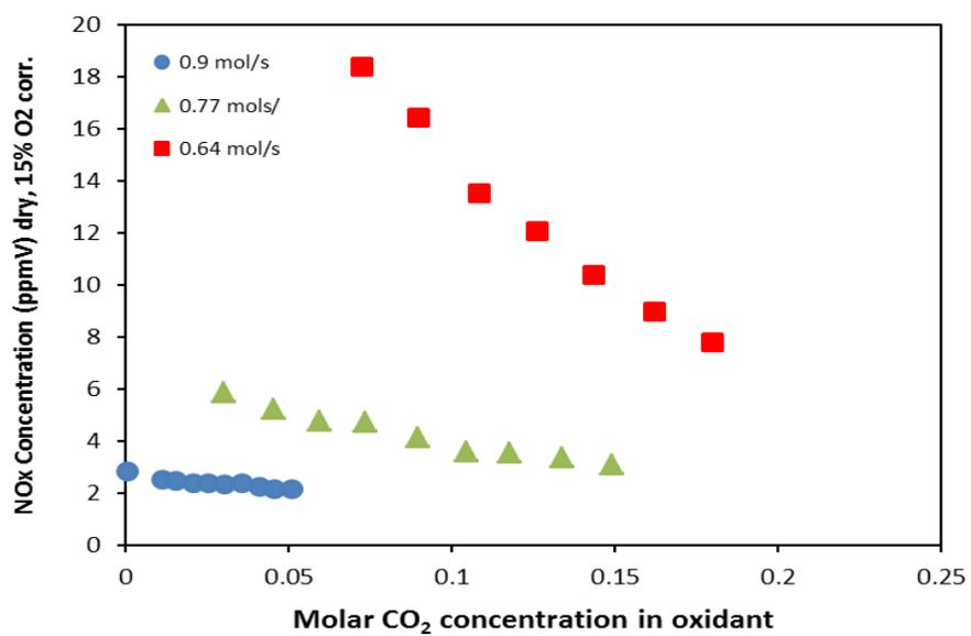
Normalised (dry 15%O<sub>2</sub>) NO<sub>x</sub> concentrations for each flow and CO<sub>2</sub> condition at 42 kW, 1.1 bar<sub>a</sub>.
