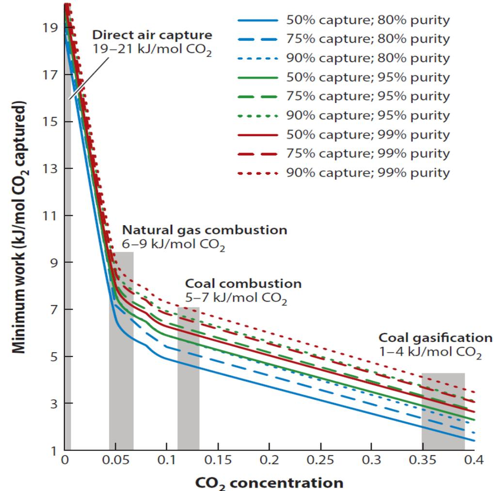
Minimum work required for  $\text{CO}_2$  capture based upon initial gas concentration, percent capture, and final purity of  $\text{CO}_2$ .
