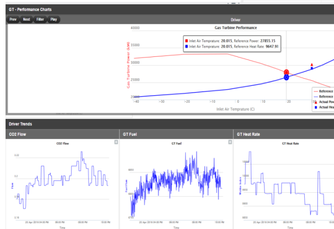
Figure 9: Example gas turbine Level 2 performance trends
