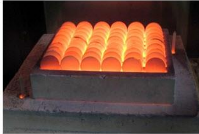
60 FCT Buttons Tested in Per Run
