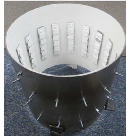
Low k TBC Coating on Property Validation Test Specimens
