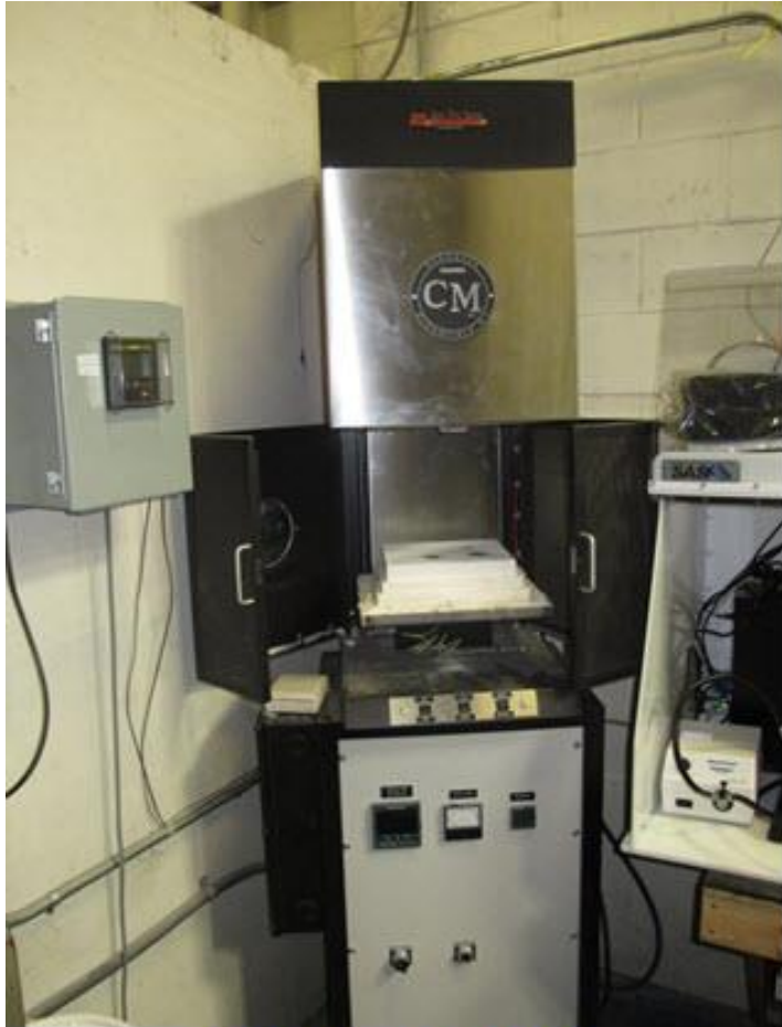
CTS Furnace Cycle Test
