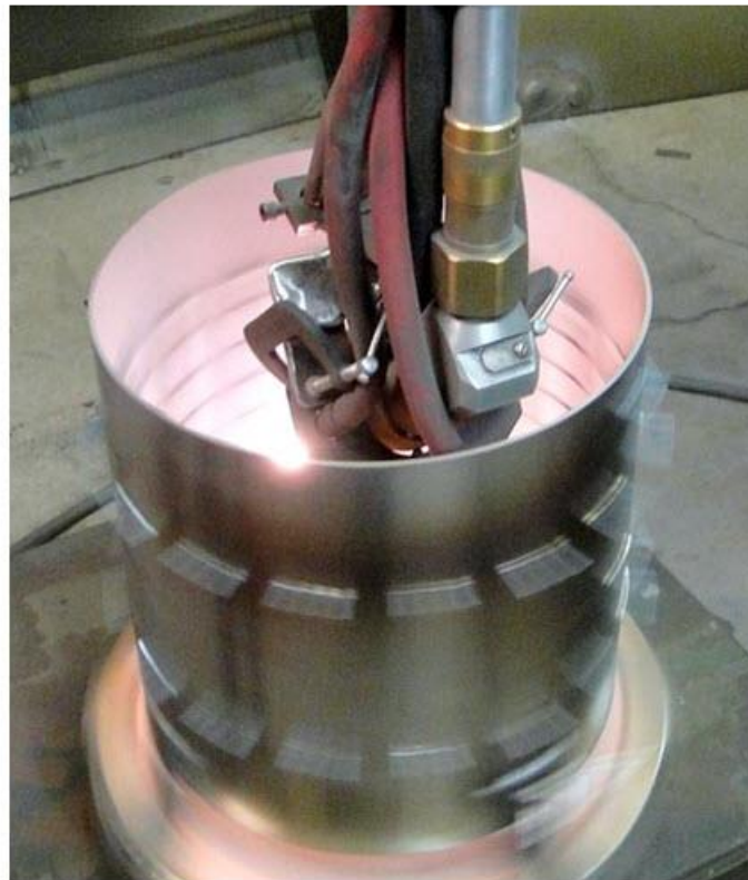
Low k TBC Coating on Property Validation Test Specimens
