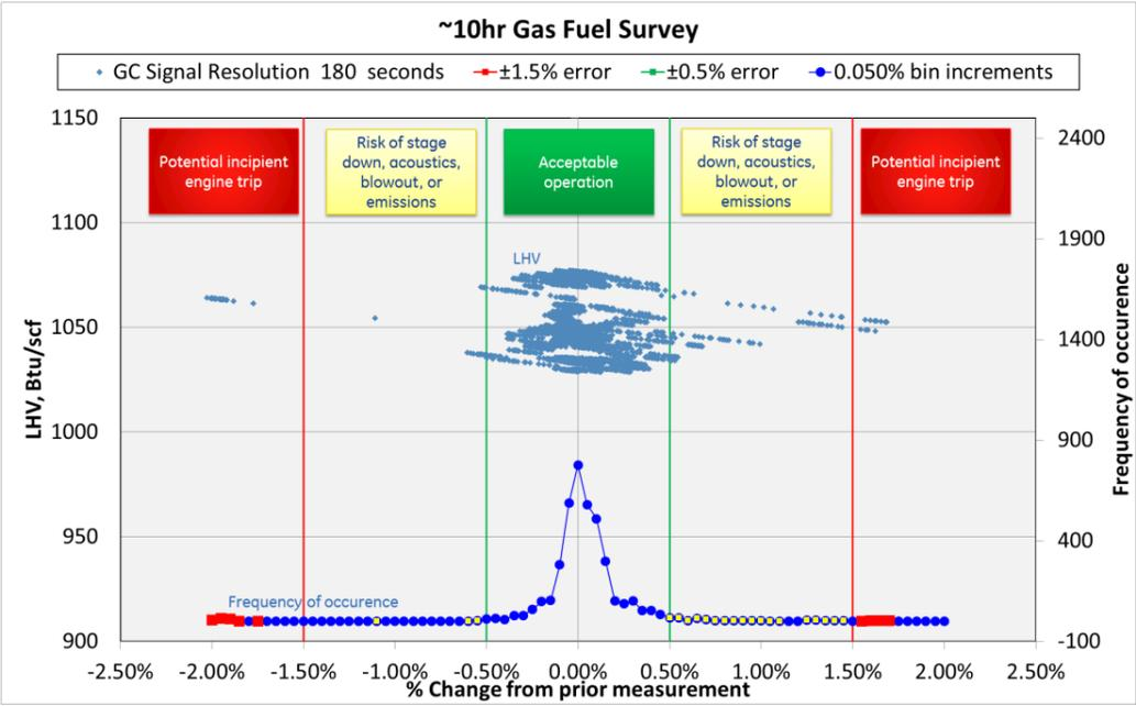
Figure 5 - GC LHV resolved by percent change in adjacent measurements during the fuel survey
