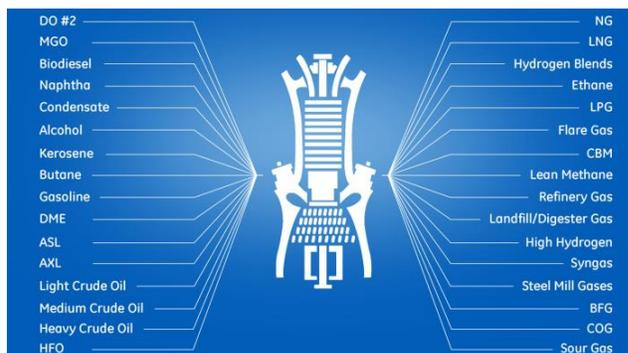
Figure 2 - GE gas turbine fuel capabilities
