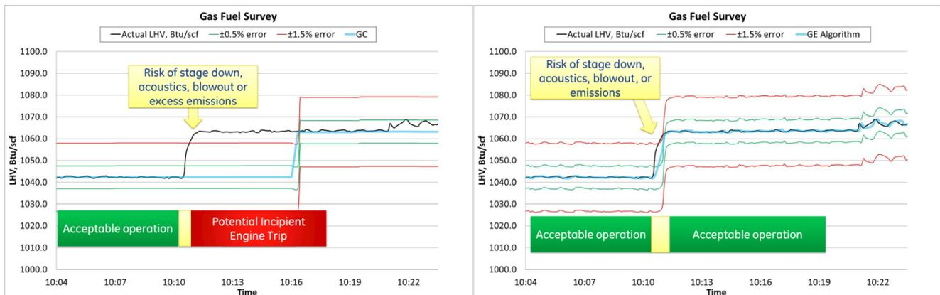
Figure 4 - Comparison of lagging GC signal and algorithm signal during a transient composition event
