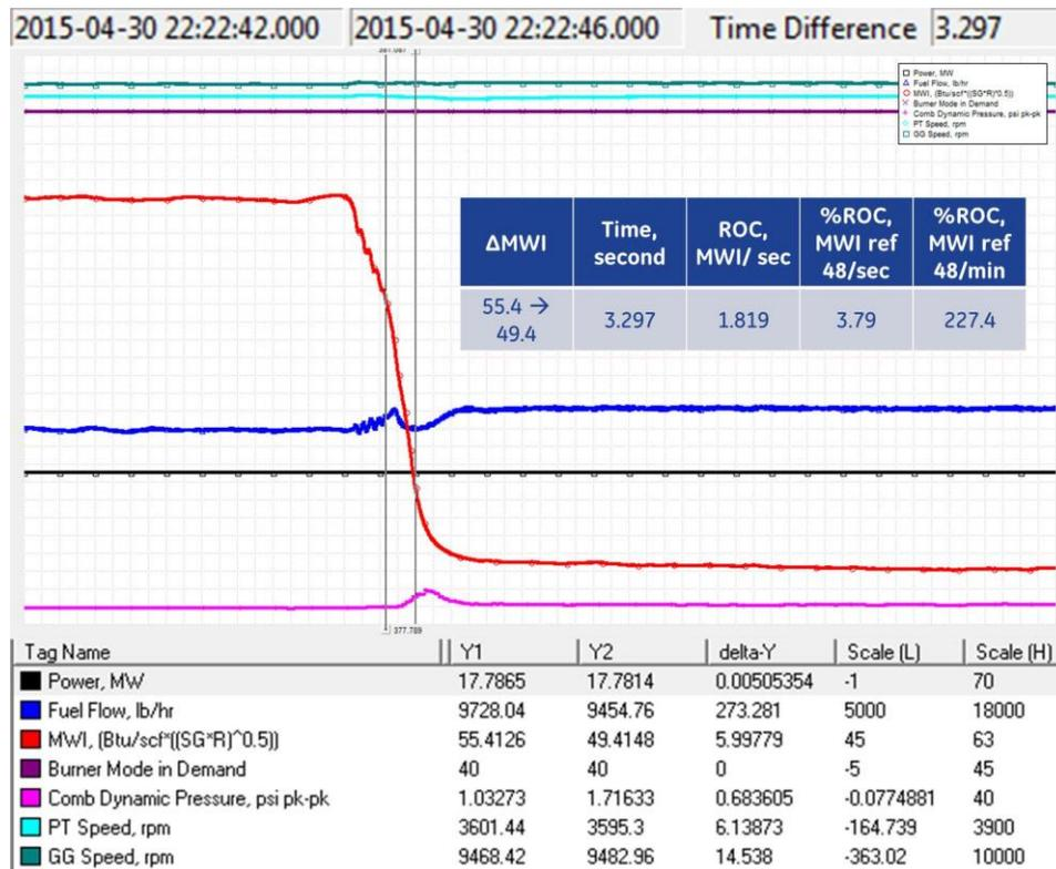
**Figure 7** - Operation at > 3.7% MWI/second rate of change on a LM2500+G4 DLE using blended natural gas and HD5 propane
