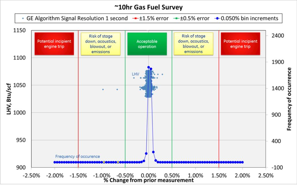
Figure 6 - Algorithm produced LHV resolved by the percent change in adjacent measurements during the fuel survey
