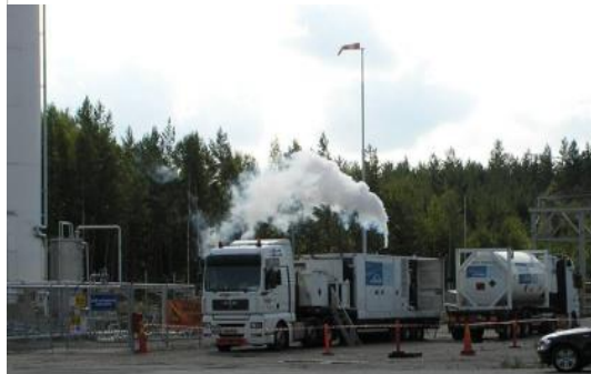
Figures 7 and 8: Measurements from SGT-700 Gas Turbine test with N 2 blending, and a photograph of the gas blending system in operation
