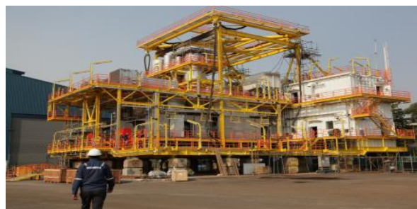
Figure 6: SGT-400 Generator Set modules for an Offshore Platform, South-East Asia, configured to run on two different fuel gases, one with a high CO 2 content
