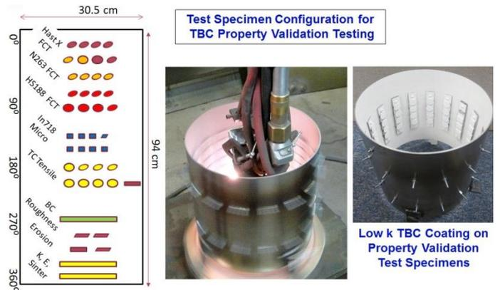
**Figure 3 Thermal Spray Configuration for Combustion Hardware Property Validation Test Specimens.**
