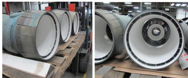
**Figure 7 Combustion Baskets – As Coated**
