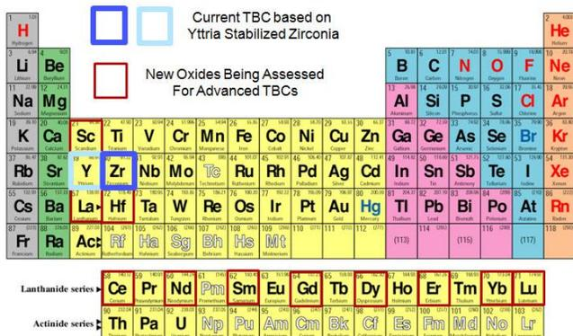
**Figure 1 Periodic Table of the Elements Highlighting New Oxide Composition Elements Being Evaluated for Low k TBCs.**
