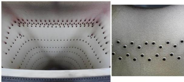
**Figure 13 Transition Piece S/N 178 Visual Appearance of TBC after engine test**
