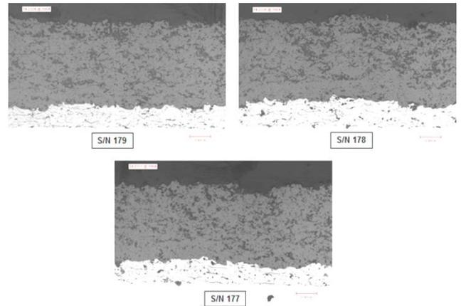
**Figure 10 QC results for Combustion Baskets – As Coated Microstructures**
