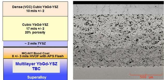
**Figure 16 Schematic of Multilayer YbGd-YSZ TBC and Photomicrograph of Multilayer YbGd-YSZ TBC**
