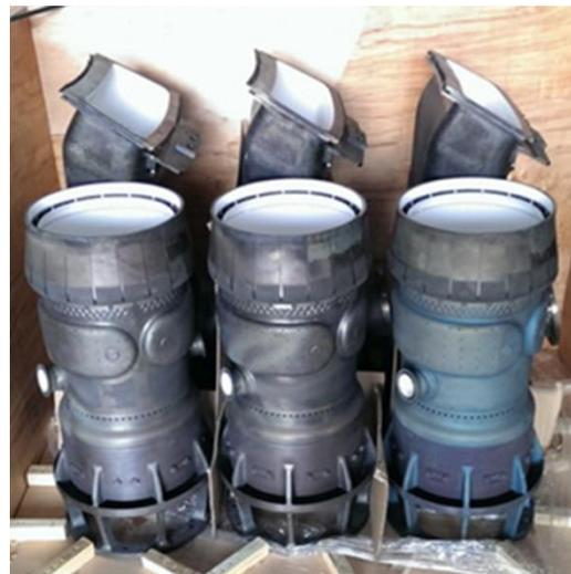
**Figure 11 Combustion Transition Pieces and Baskets coated with CT 1702 low k TBC system Ready for Shipment**
