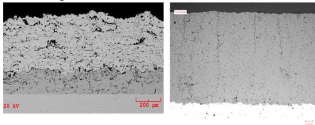
**Figure 15 Photomicrograph of Baseline 7YSZ Porous TBC 10-15% porosity (left) and Baseline 7YSZ VCC TBC**
