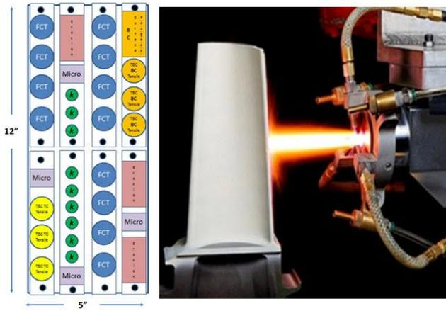
**Figure 14 Airfoil TBC Program Thermal Spray Specimen Layout (left), IGT Airfoil being Coated with a TBC (right)**
