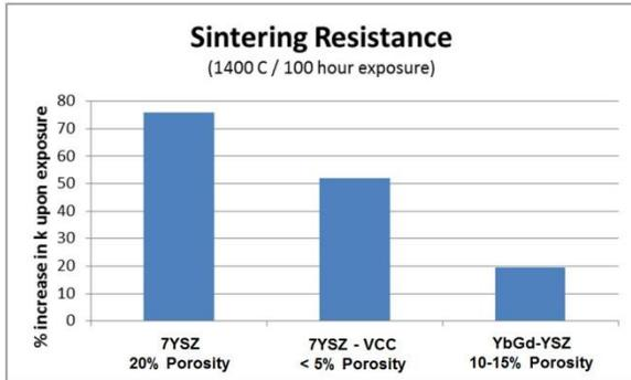
**Figure 5 Increase in Thermal Conductivity for 7YSZ compared to YbGd-YSZ TBCs following a 1400 C / 100 hour thermal exposure**
