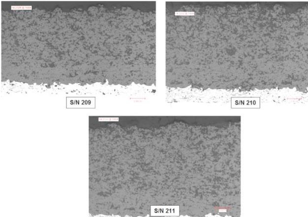
**Figure 8 Task 3 QC results for Combustion Baskets – As Coated Microstructures**
