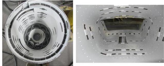
**Figure 6 Test Tab locations used to qualify the CT1702 Coating Process on a Scrap Combustor Basket (left) and Transition Piece (right)**
