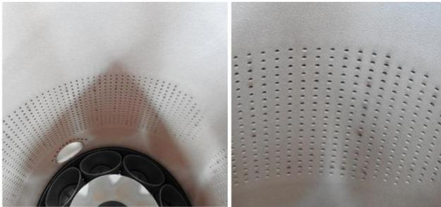
**Figure 12 Basket Visual Appearance of TBC after engine test**
