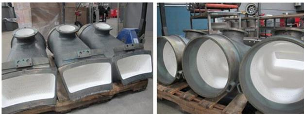
**Figure 9 Combustion Transition Pieces– As Coated**
