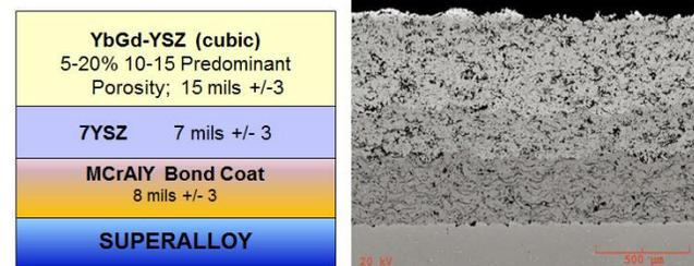
**Figure 4 CTS CT1702 low k dual ceramic layer 7YSZ/YbGd-YSZ TBC coating system**
