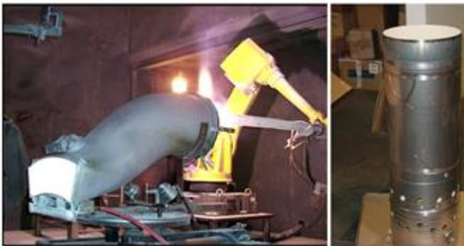
**Figure 2 Transition Duct being Plasma Sprayed with a TBC (Left) and a TBC Coated Combustion Basket (right). (Courtesy of CTS)**
