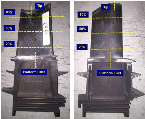
**Figure 17 Metallographic Sectioning Plan for Qualifying Baseline and Low Multilayer TBCs on F Class Stage 1 turbine Blades**
