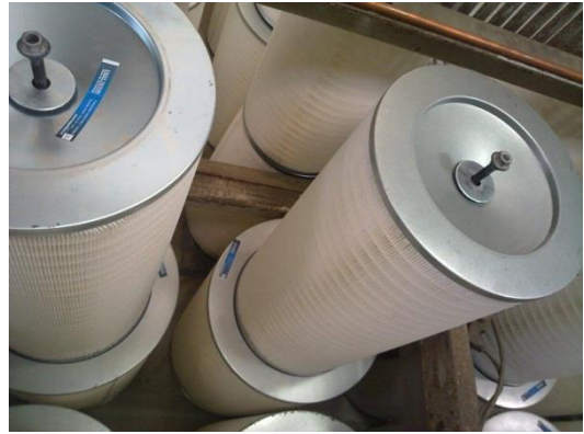
Figure 12. EPA-2 Main filter during installation
