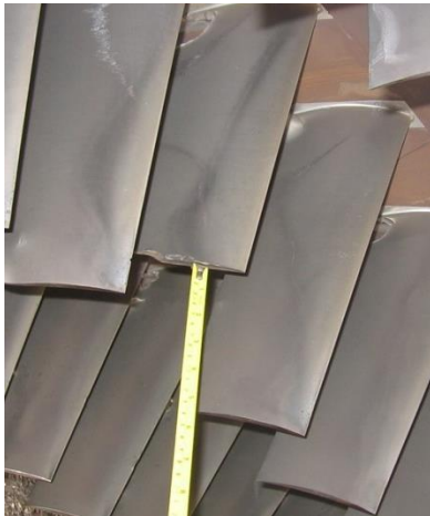
Figure 6. Broken compressor stage No. 1 stator blade: loss of the blade tip (~25% of the blade height).
