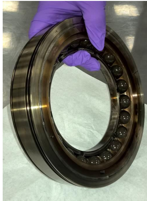
bearing with one inner ring half removed, showing the ceramic balls and the cage
