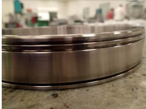
outward outer ring featuring piston ring grooves for squeeze film damping
