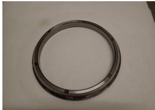
loaded inner ring with radial oil slots in the split face
