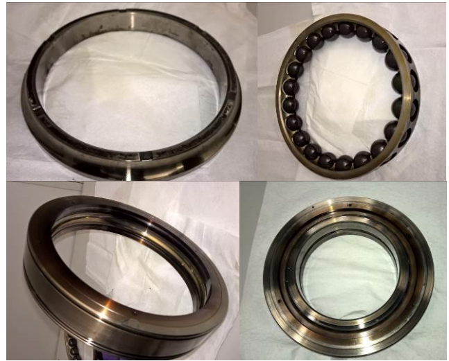
Fig. 3: Rig tested components of the investigated hybrid ball bearing: inner ring half (top left), cage/ball assembly (top right), outer ring (bottom left) and bearing assembly (bottom right)
