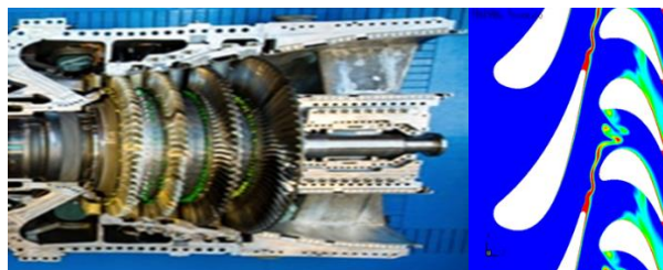
Figure 7. 7/9HA Turbine (left) and velocity field from computational fluid dynamics (right)
