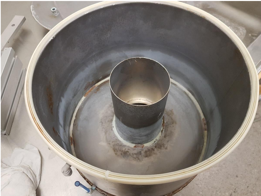
FIGURE 6. SALT WATER CONTAINER WITH EXIT PIPE IN THE MIDDLE. PIPE CUT TO 170MM.
