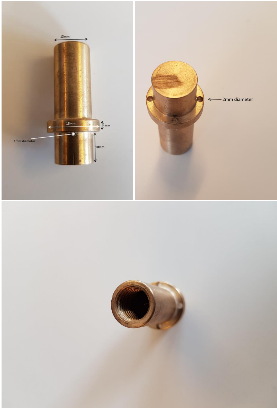
FIGURE 4. DIMENSIONS OF LASKIN NOZZLE
