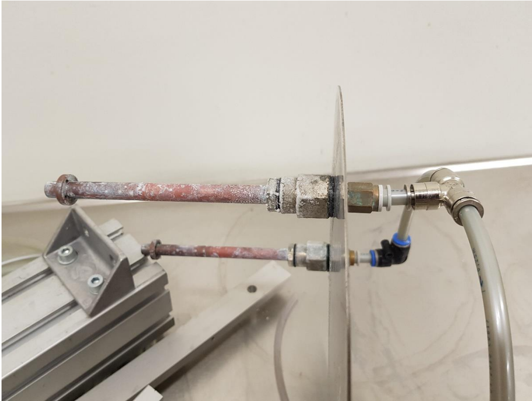
FIGURE 5. ATTACHED LASKIN NOZZLES TO TOP LID SHOWING CONNECTORS ETC. MK.II SHOULD BE STAINLESS.
