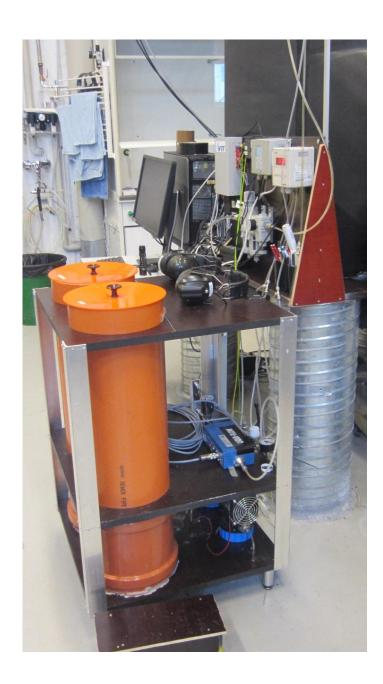
←Salt water container, pump and mass flow controller for the salt water flow control
