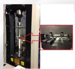
RT an HT 4 point bending test ASTM C1161-13&C1211-13
