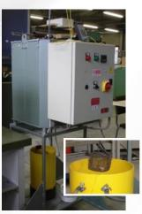
Thermal shock ASTM C1525-04
