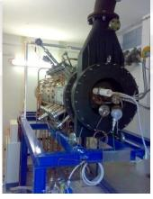
The rig is typically operated using natural gas, but even non-conventional gas mixtures, such as Hydrogen Rich Syngas Low-BTU gases, Biogas may be tested
