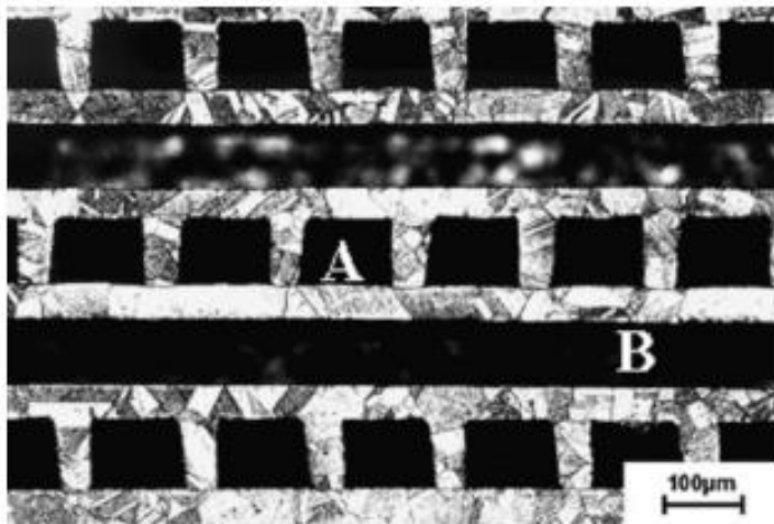
Fig. 2. Optical micrograph of a plane cut through a stainless steel
