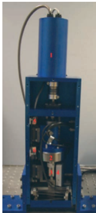
Figure 1: DNV KEMA's indentation test device measuring actual material properties.
