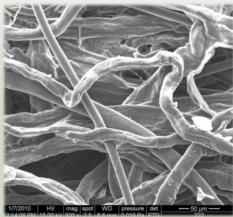
Typical filtration media for Pulse-jet filters
