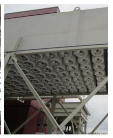
System loss due to fouling using F7/MERV 14 canisters is 10% over 2200 hours.
