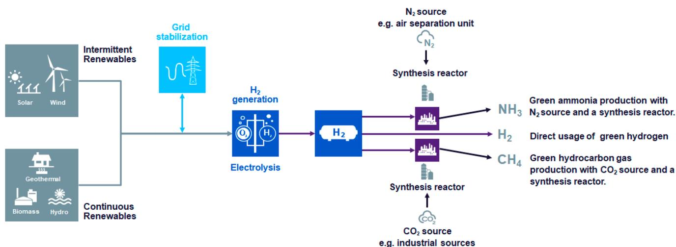
Figure 4: Simplified process flow diagram for power-to-gas applications
