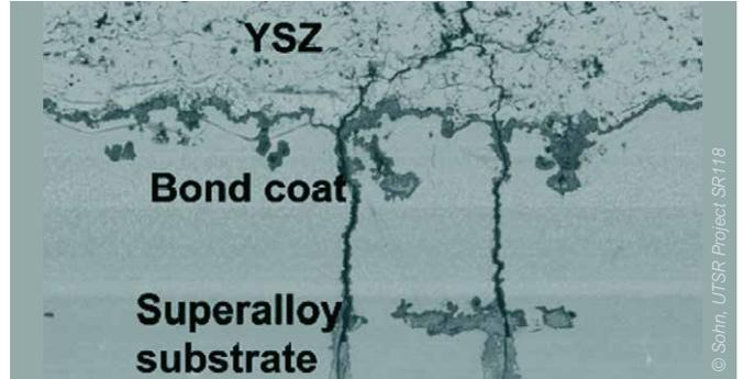
Figure 10: Scanning electron micrograph of cross-section of coated blade material expose in a combusted syngas environment showing deposit penetration
