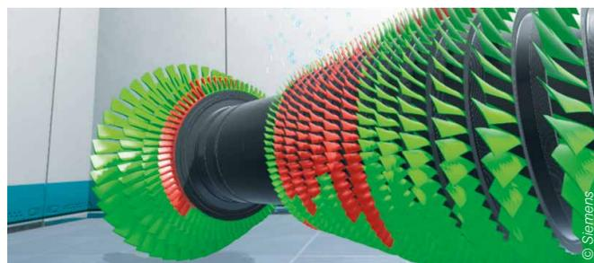
Figure 13: In a virtual reality representation of a gas turbine, complex sensor data is translated into colors to make the meaning of information in this case temperature differences easy to understand
