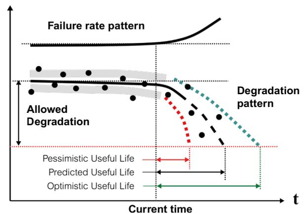
Figure 12: Degradation and prognostic model
