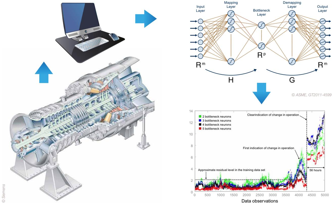
Figure 17: Collecting data and using a neural network for condition monitoring and early detection of upcoming faults
