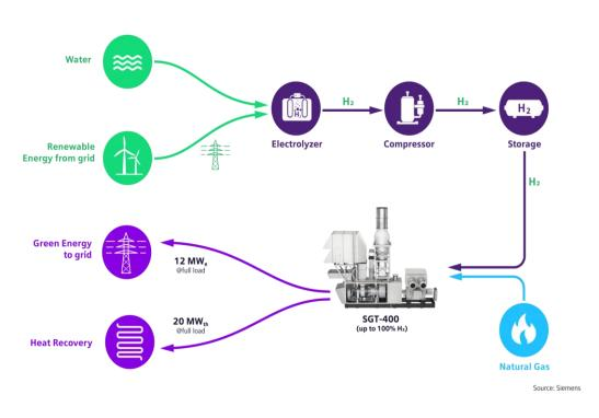
Smurfit Kappa plant in Saillat-sur-Vienne, France: Pilot Cogeneration SGT-400 Plant
