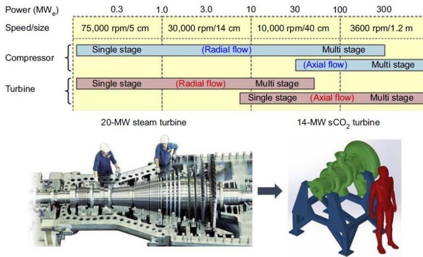
Figure 2 - Size of the sCO<sub>2</sub> turbomachinery as a function of power and speed [2].
