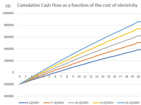
Figure 22 - Cumulative cash flow as a function of the cost of electricity
