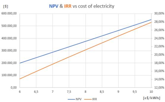
Figure 8 - NPV & IRR vs cost of electricity
