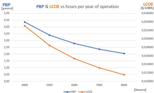
Figure 18 - PBP & LCOE vs hours per year of operation
