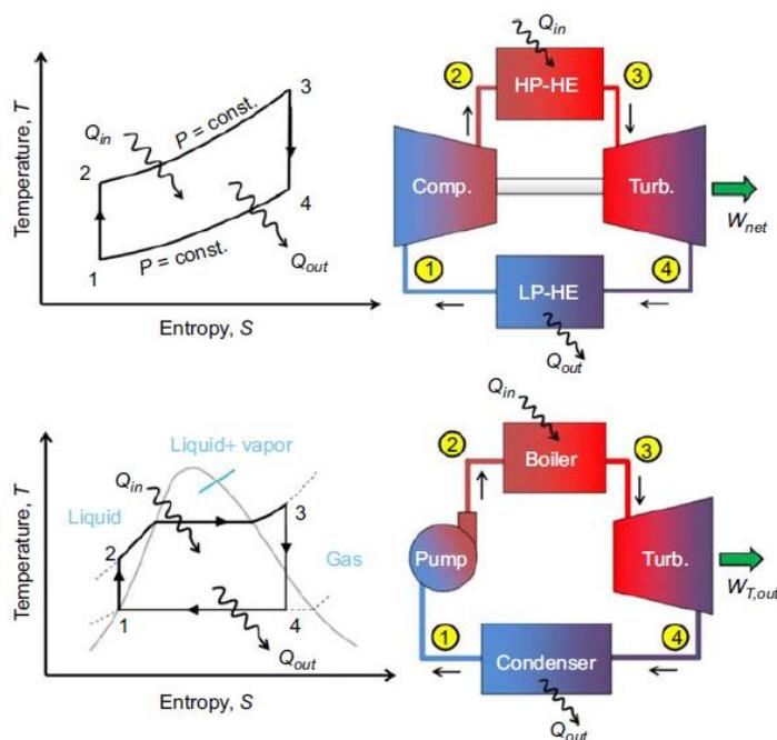
Figure 1 - Brayton and Rankine cycles (up and down respectively in the illustration) and relative plant components
