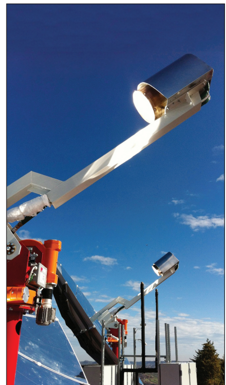
Each unit has its own MGT, which sits on an arm attached to the solar dish.
