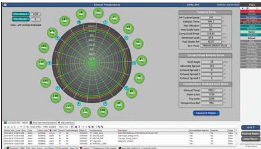
Swirl chart displays. These help operators identify the location of malfunctioning combustion hardware in gas turbines.
