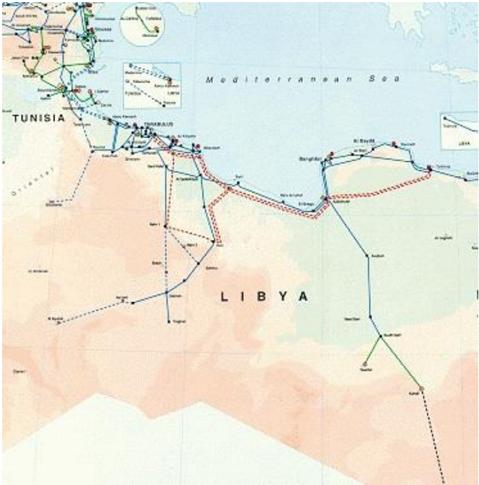
Figure A. 54. Lybia electricity grid.
