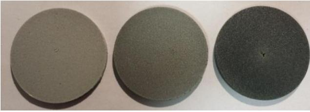
**Figure 10. Samples of paint applied to Inconel substrates then heated at 800°C (left), 900°C (middle) and 990°C (right) for 30 minutes.**
