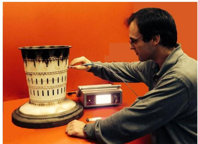
**Figure 1. An operator using the measurement equipment is contained within a box with a fibre guided probe and a touchscreen for control.**
