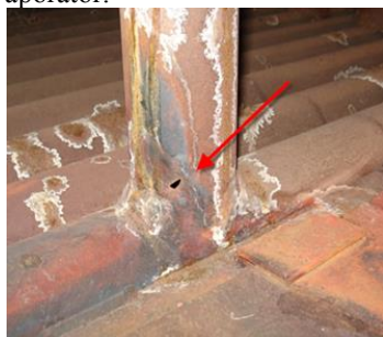
Figure 1: Hole caused by FAC on connection of LP evaporator outlet header
